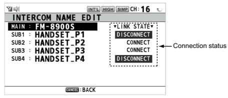
3. Rotate the CHANNEL/ENTER knob to select the terminal then push the knob.
